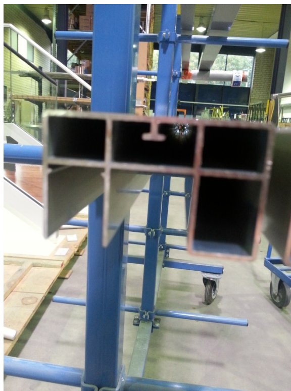
Plate 2 – Internal Profile Square Hand Rail
